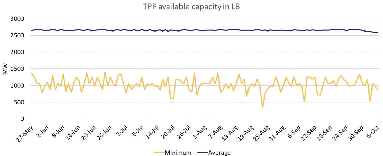
**Figure 29 Average and minimum TPP available capacity in Lebanon.**
