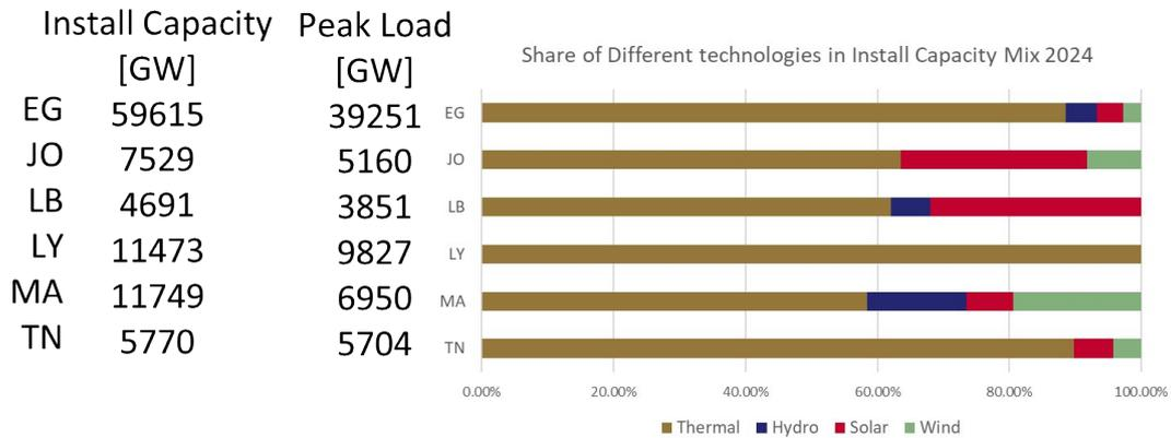
**Figure 13 Install capacity mix and peak load in 2024.**
