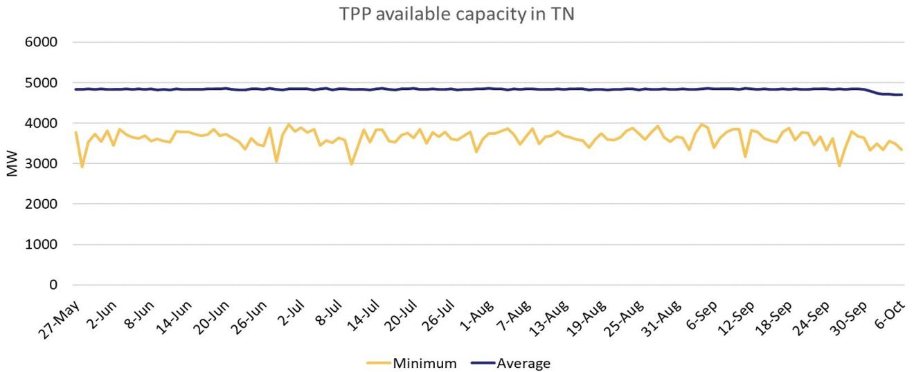
**Figure 44 Average and minimum TPP available capacity in Tunisia**
