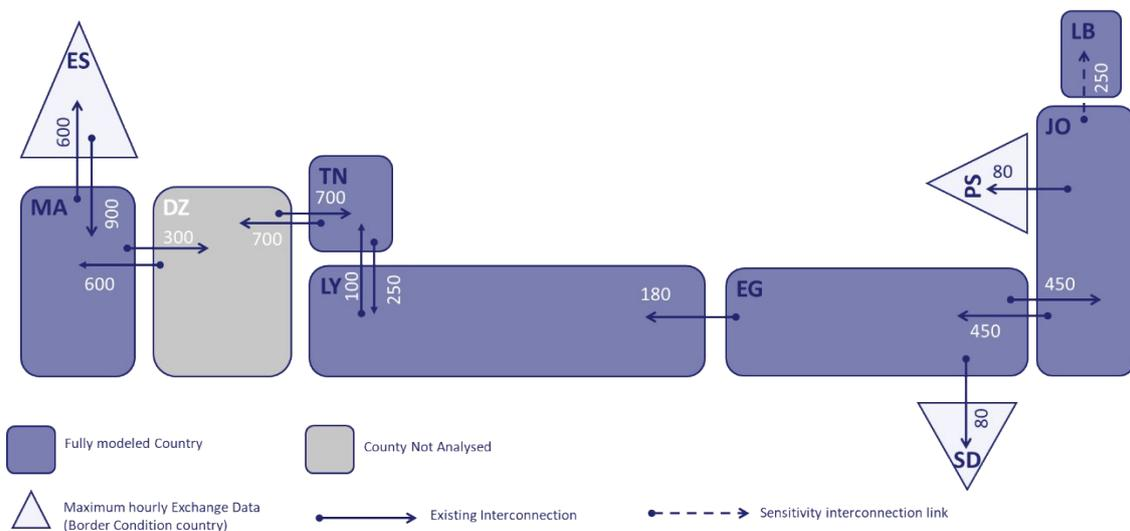
Figure 14 Net Transfer Capacity during SO2024
