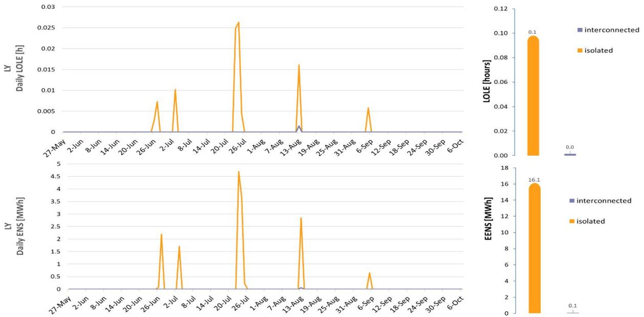
**Figure 36 Daily LOLE and EENS for the interconnected and isolated mode of operation in Libya.**
