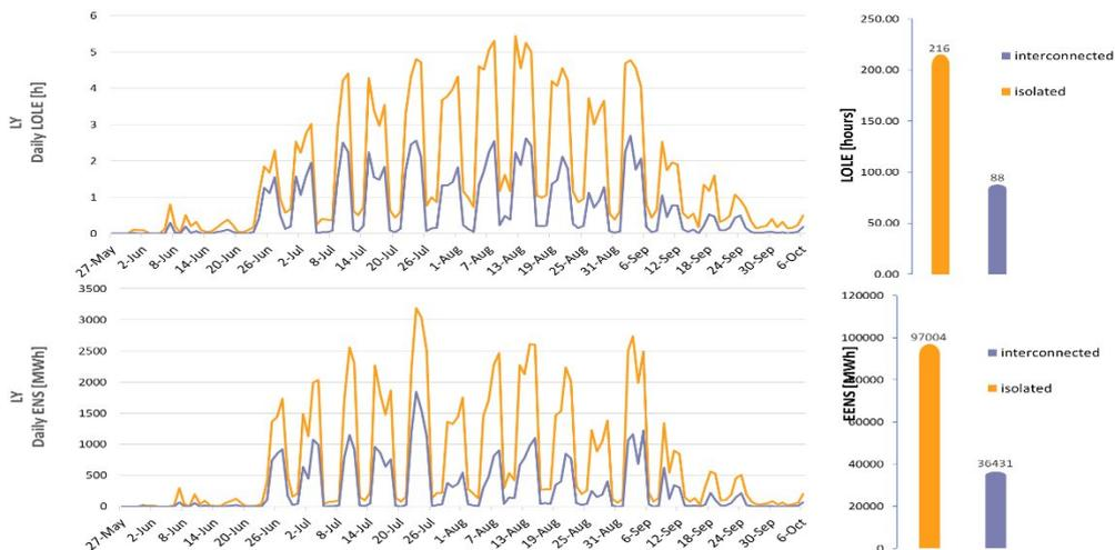
**Figure 54 Daily LOLE and EENS for the interconnected and isolated mode of operation in Libya.**
