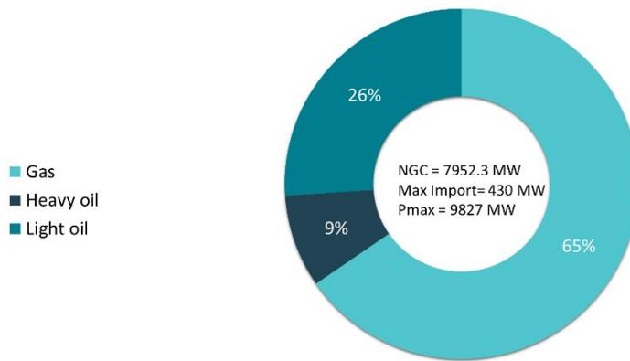
**Figure 51 Installed Capacity mix with total NGC, import NTC and peak demand in Libya (Sensitivity Case).**
