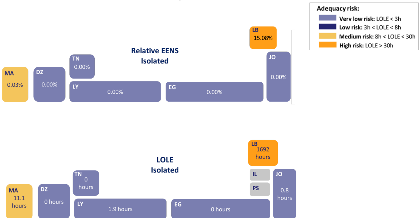
Figure 16 Seasonal Relative EENS and LOLE for the isolated mode of operation for only winter season
